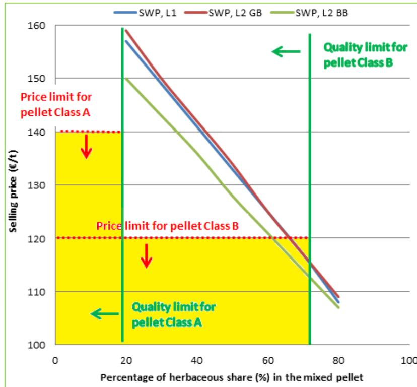
**Figure 6: Limits in quality and price for Class A and Class B and confort zone.**
