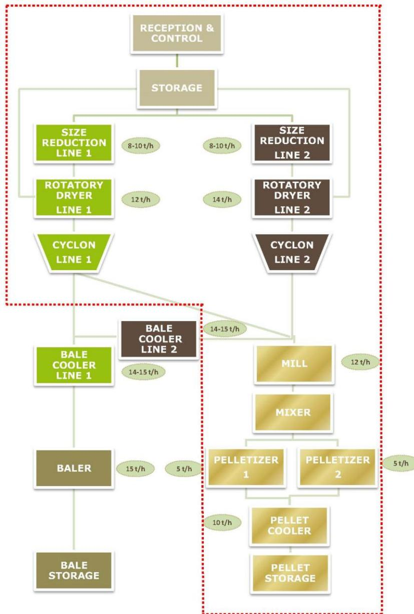
**Figure 3: Flow diagram of the current alfalfa production lines (equipment proposed for the biomass logistic centre surrounded in red).**
