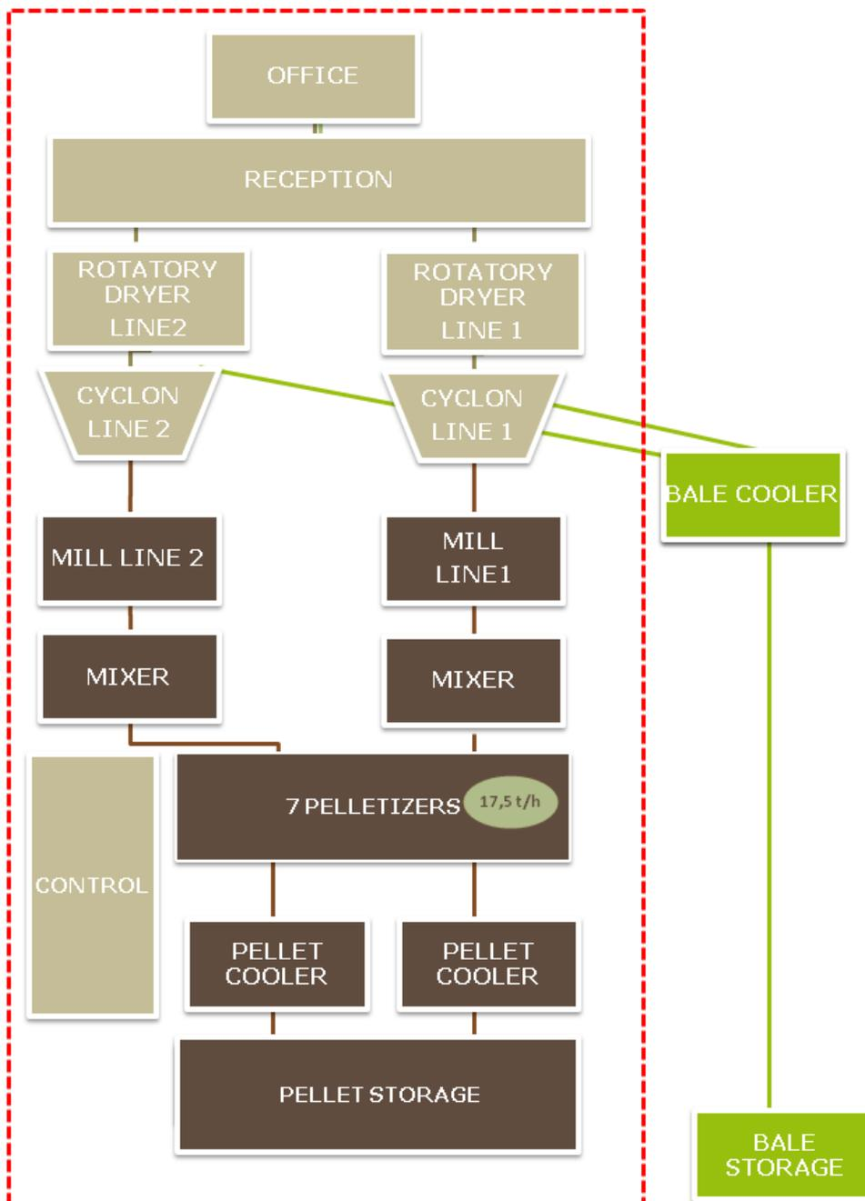
Figure 7: Flow diagram of the current alfalfa pellet production lines.
