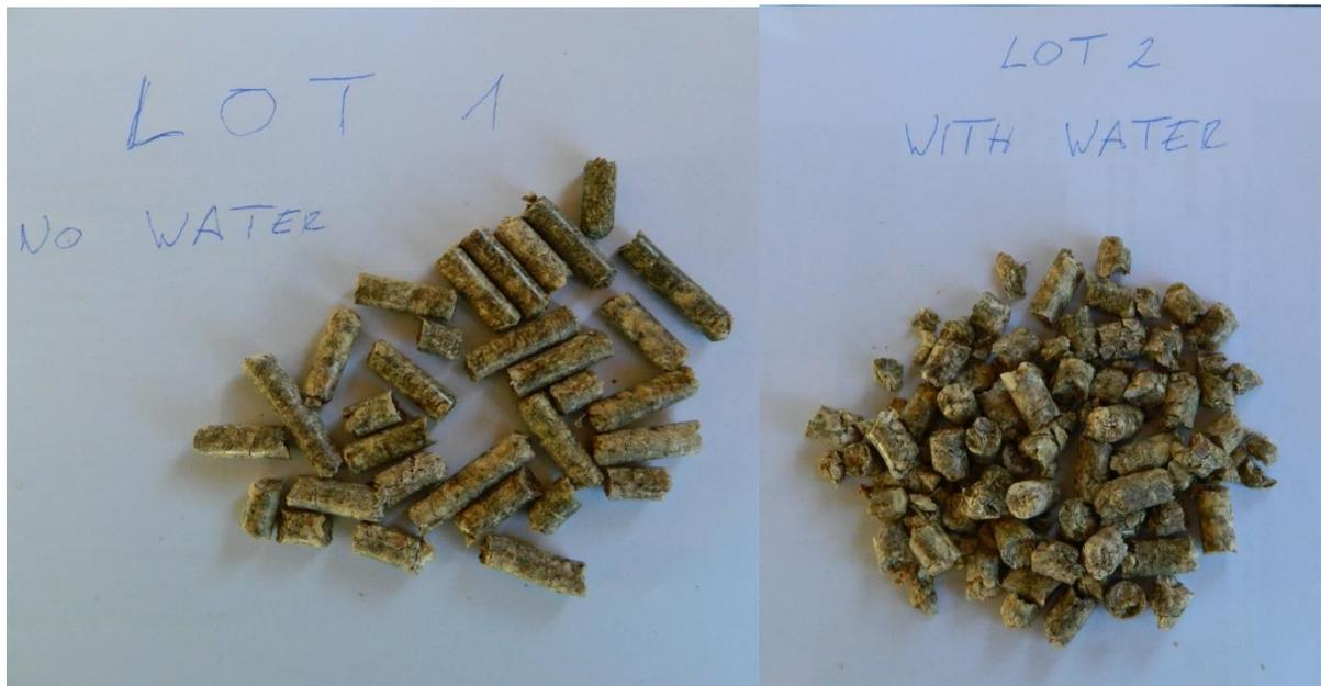
**Figure 1: Sample pellets with and without steam**
