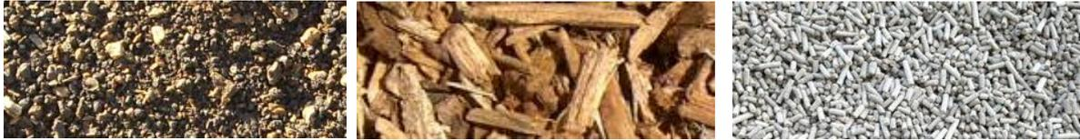
**Figure 9 : Different formats of biomass provided by the company Daniel Espuny (from left to right: pulverized olive pomace – pruning wood chips – pelletized olive pomace)**
