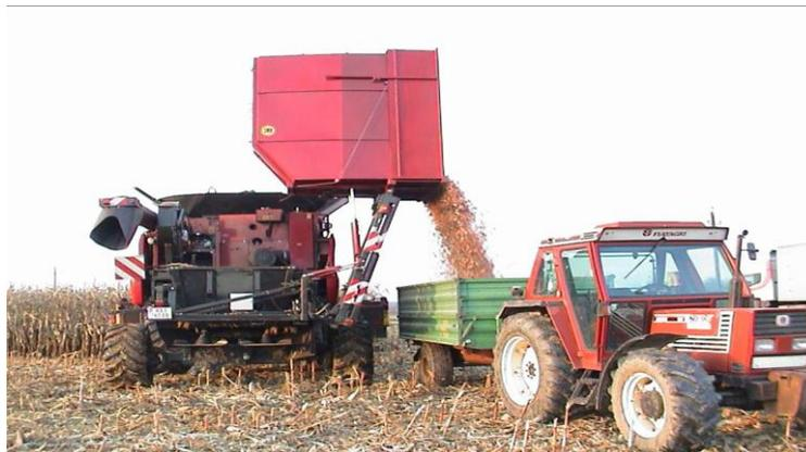
Figure 5 : Tschiggerl Agrar corn cobs harvester
