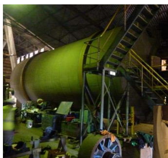
Figure 4 : Horizontal dryer – Luzéal - France
