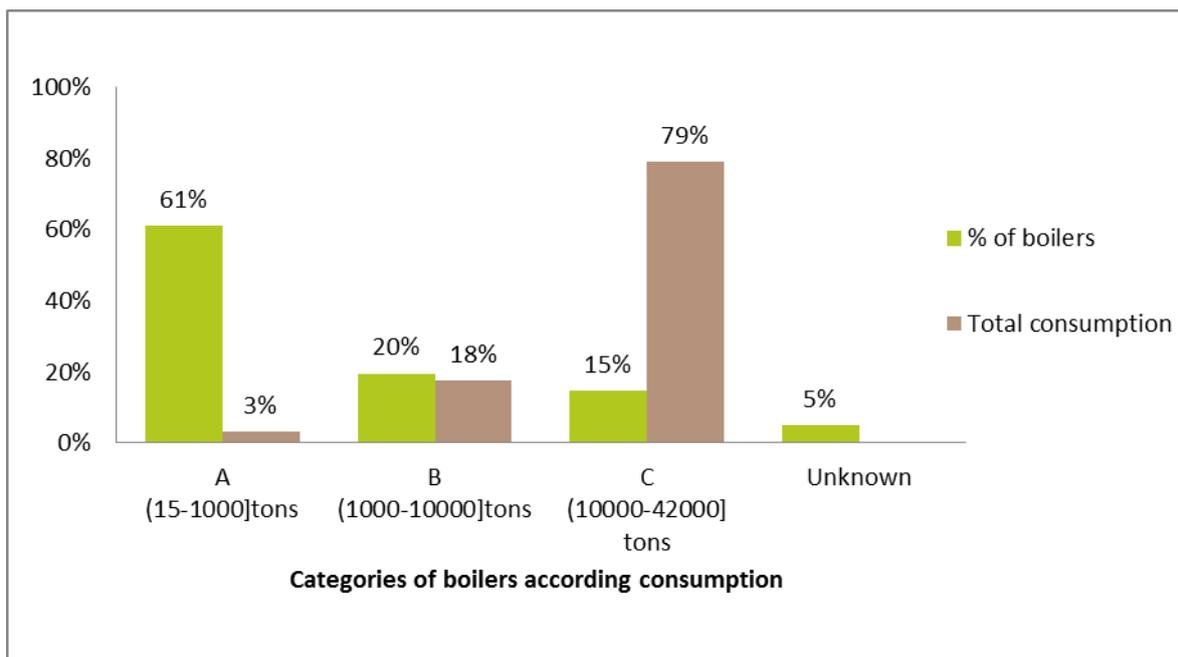
**Figure 6: Boiler classes and share of consumption (Source: UCFE-GCF).**
