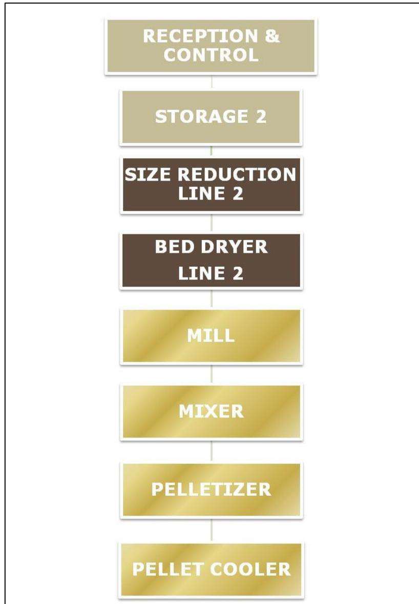
**Figure 1: Scheme of logistic centre manufacturing processes**
