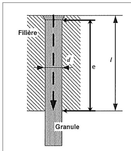
**Figure 4: Structure of a die**
