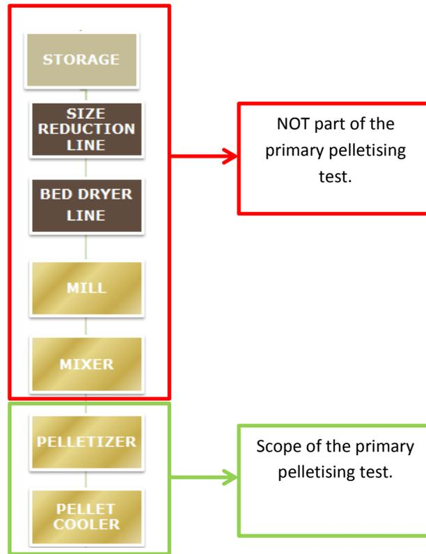
Figure 5: process first production test
