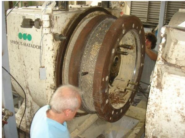
**Figure 3: Die and pelletiser of Tschiggerl Agrar (Austria)**
