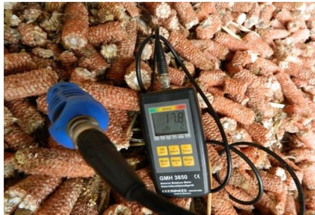
**Figure 17. Moisture checking in raw material**
