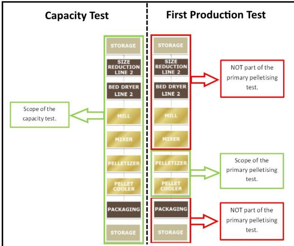
Figure 11: Comparison capacity test vs. first production test
