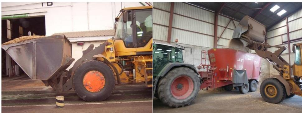
Figure 6: Manual mixing of raw materials
