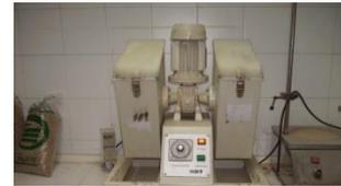
**Figure 2: Durabilimeter**
