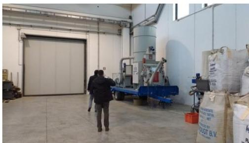
**Figure 7:** pelletizing line (movable-for field use) for agrarian pruning – Costruzioni Nazzareno
